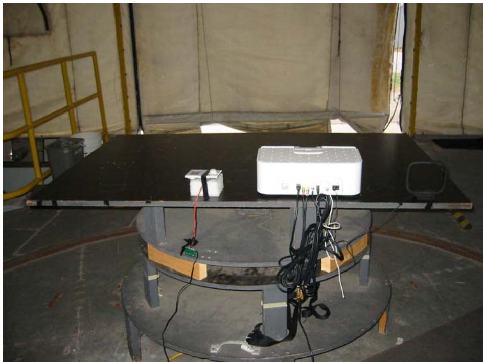
**Test Results:** Pass**Test Standard:** FCC Part 15 Subpart B & C**Test:** Line-conducted emissions**Performance Criterion:** Readings below specified limits**Test Environment:**
