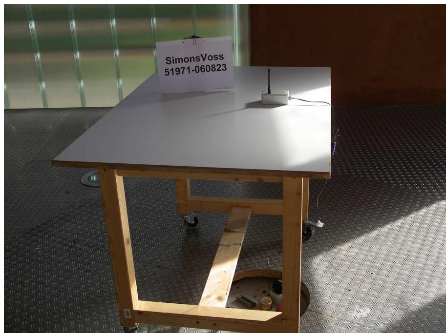
**Test setup for radiated emission measurement
