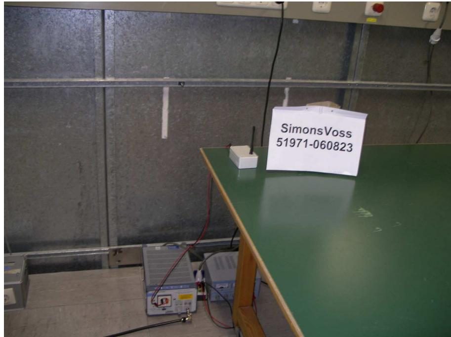
**Test setup for radiated emission measurement
