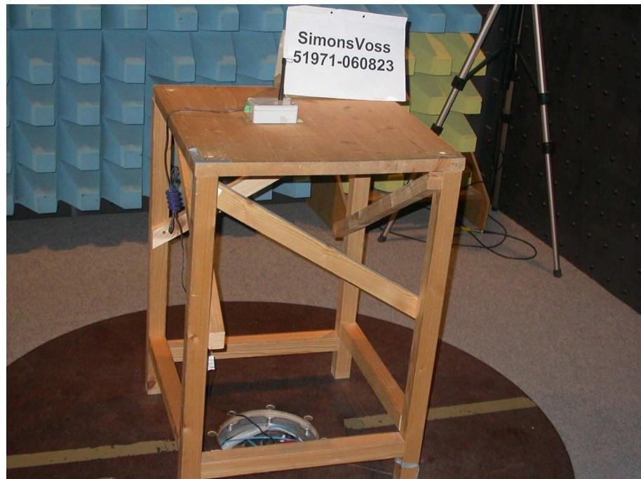
**Test setup for radiated emission measurement
