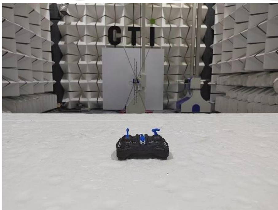
Radiated emission Test Setup-2(close up) (30MHz~1GHz)
