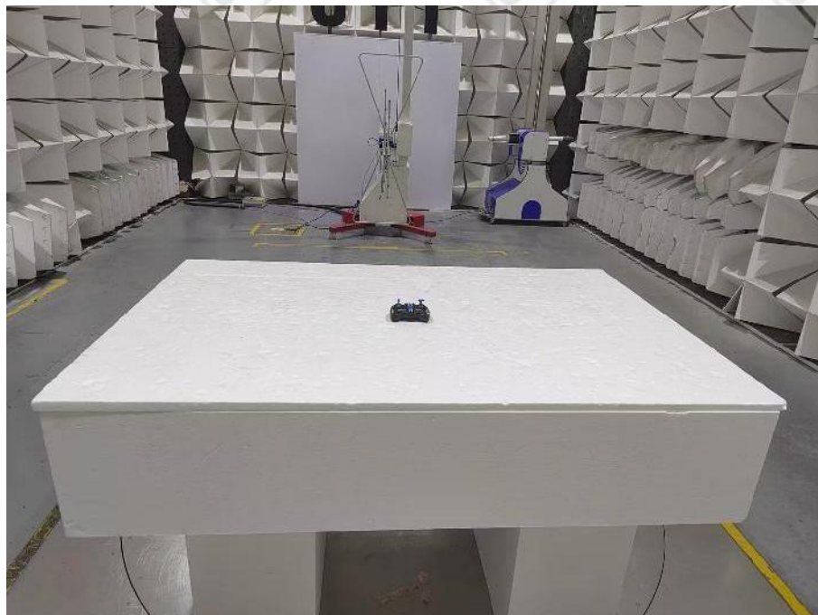
Radiated emission Test Setup-1 (30MHz~1GHz)
