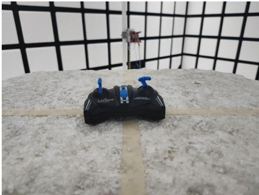
Radiated spurious emission Test Setup-3(Above 1GHz)
