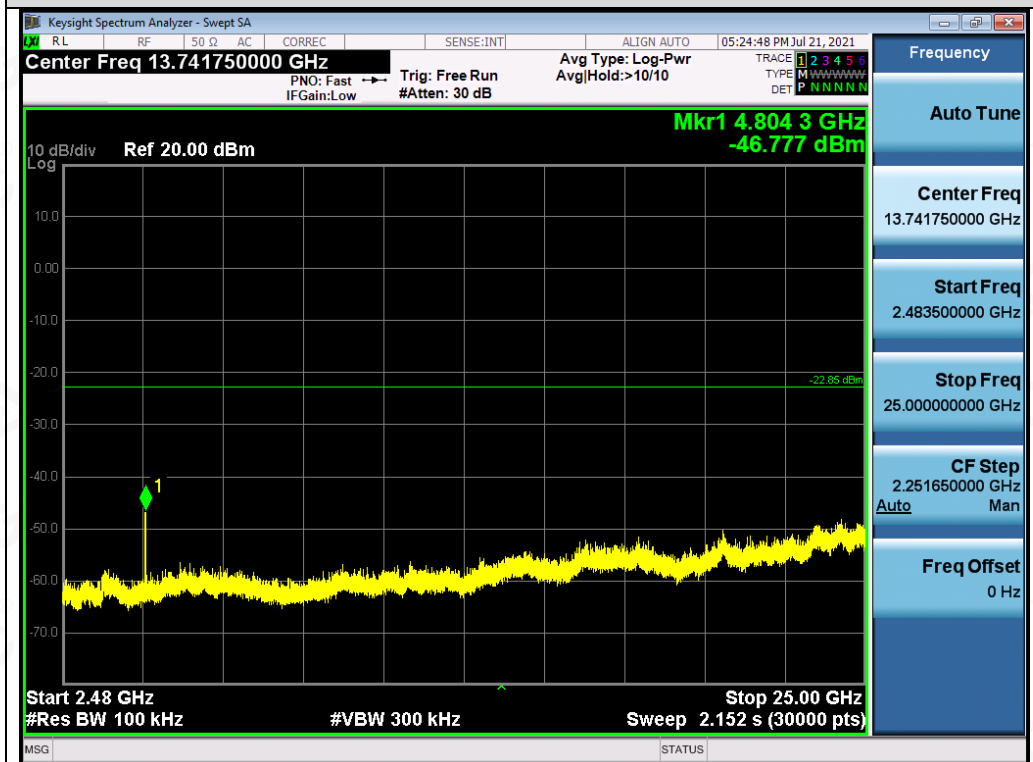
Test_Graph_EDR_ANT1_2402_2Mbps_Higher Band Emissions
