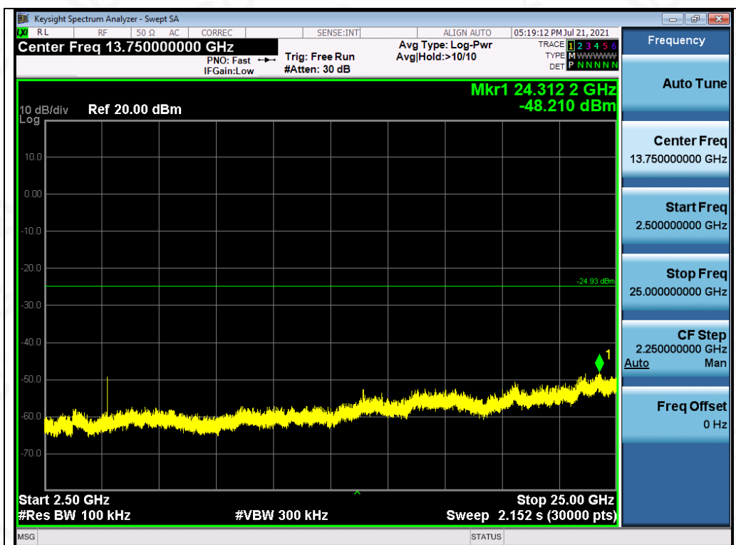
Test_Graph_BR_ANT1_2480_1Mbps_Higher Band Emissions
