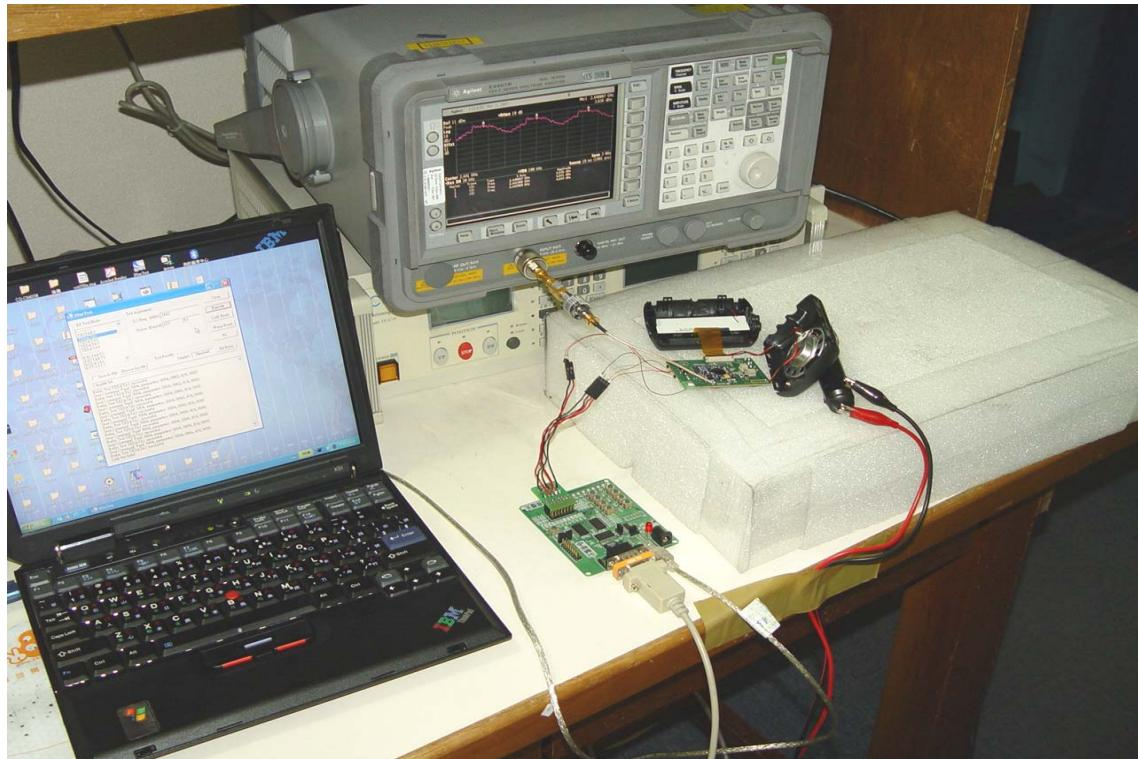
**RADIATED EMISSION SETUP PHOTOS**
