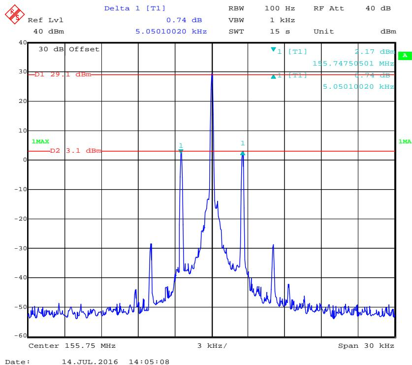
**Emission Mask E with High Power 6.25 kHz, 155.75 MHz**
