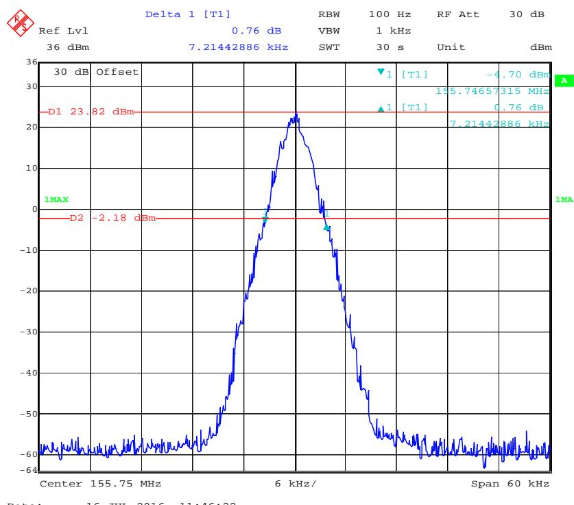
**Emission Mask D with High Power 12.5 kHz, 155.75 MHz**
