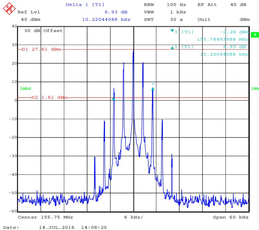
**Emission Mask D with High Power 12.5 kHz, 155.75 MHz**
