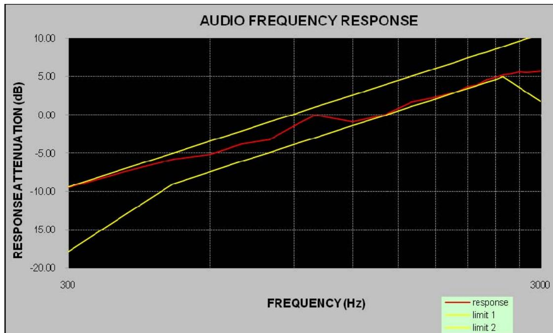
Carrier Frequency: 155.75 MHz, Channel Separation=12.5 kHz
