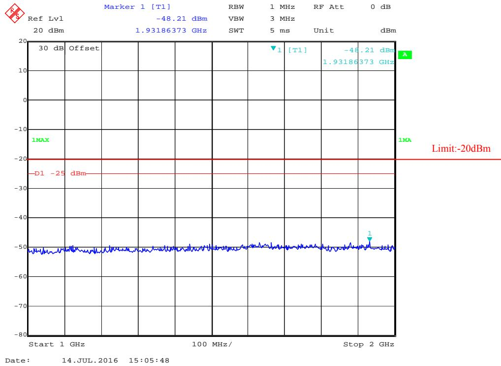
**Digital Modulation:****30 MHz – 1 GHz, Spacing Channel 12.5 kHz, 155.75 MHz**
