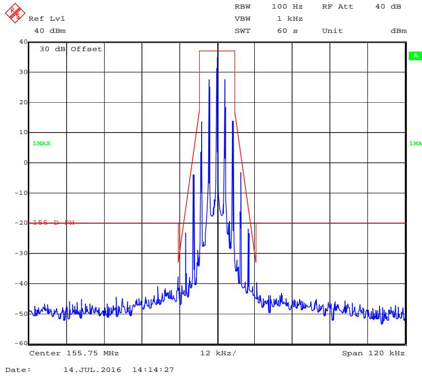
**Emission Mask D with Low Power 12.5 kHz, 155.75 MHz**
