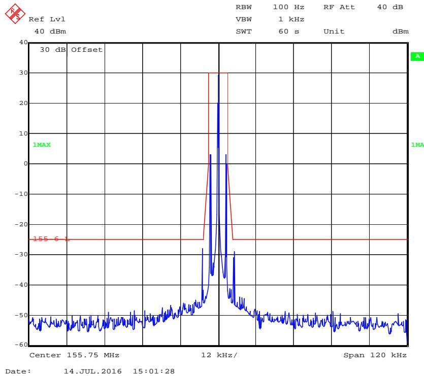
**26 dB Emissions Bandwidth 12.5 kHz, 155.75 MHz (High Power)**
