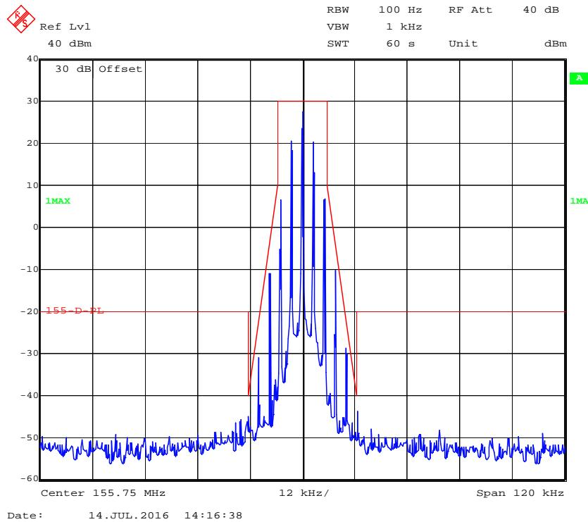
**Digital Modulation:****26 dB Emissions Bandwidth 12.5 kHz, 155.75 MHz (High Power)**
