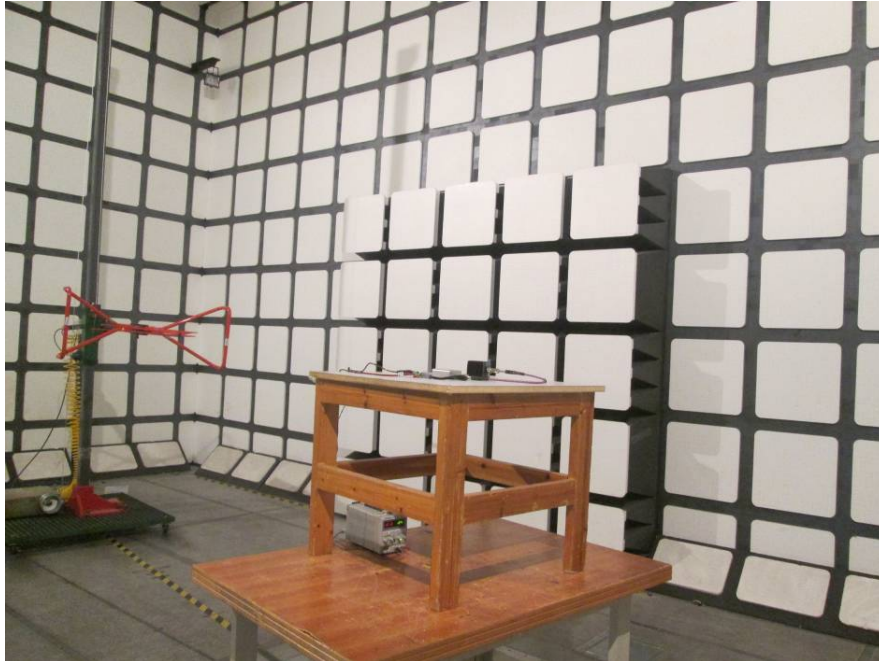
Radiated Emissions – Front View (Below 1 GHz)
