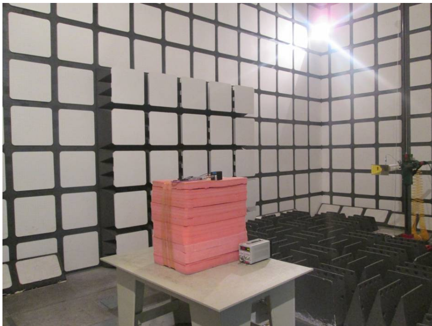
Radiated Emissions – Front View (Above 1 GHz)
