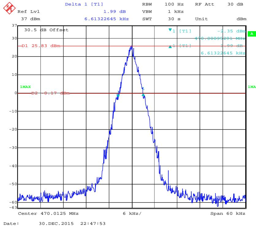
**Emission Mask D with High Power 12.5 kHz, 470.0125 MHz (4FSK (19200))**
