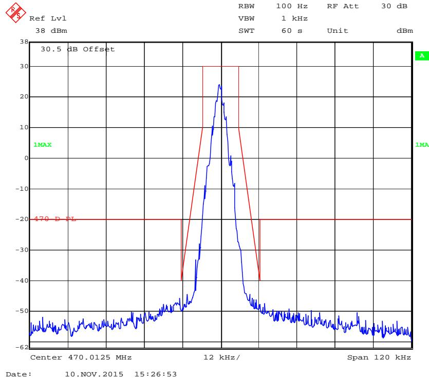
**Emission Mask D with High Power 12.5 kHz, 470.0125 MHz (4FSK (9600))**
