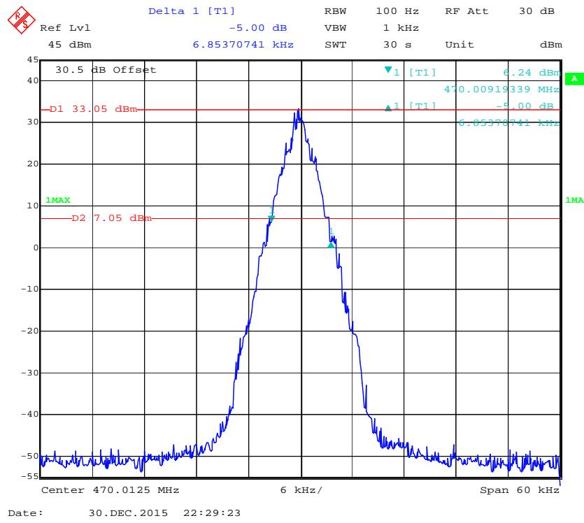
**26 dB Emissions Bandwidth 12.5 kHz, 470.0125 MHz 4FSK (9600) (Low Power)**
