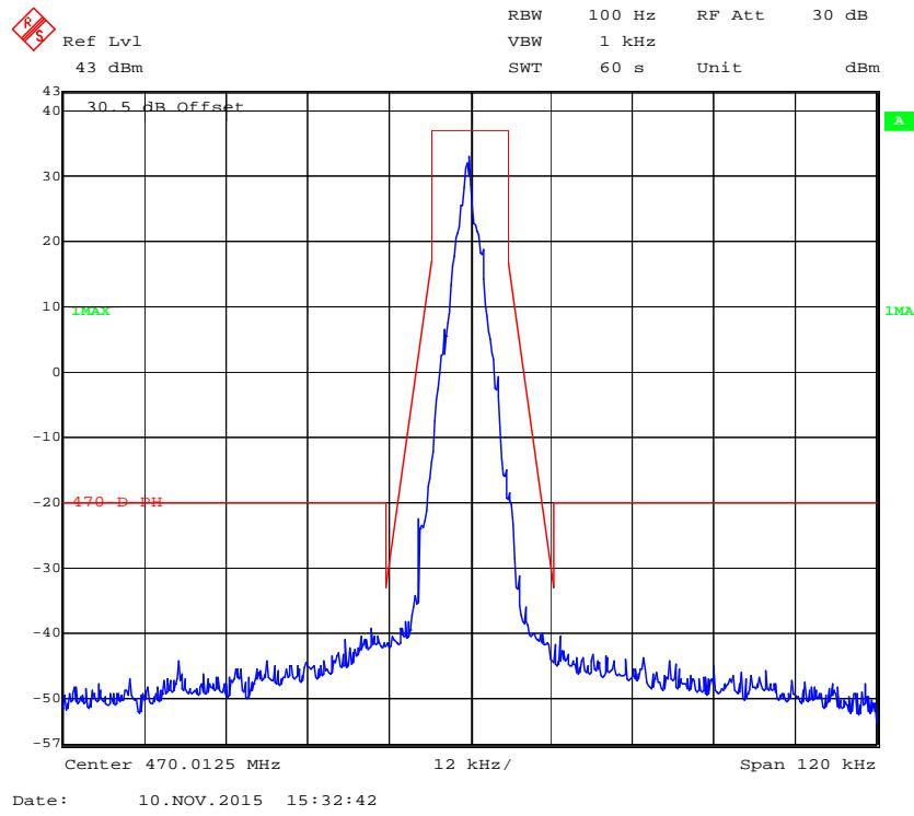
**Emission Mask D with Low Power 12.5 kHz, 470.0125 MHz (4FSK (19200))**
