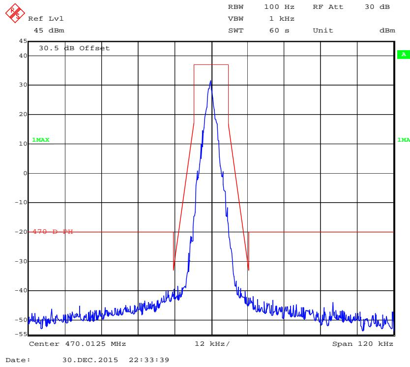
**Emission Mask D with Low Power 12.5 kHz, 470.0125 MHz (4FSK (9600))**
