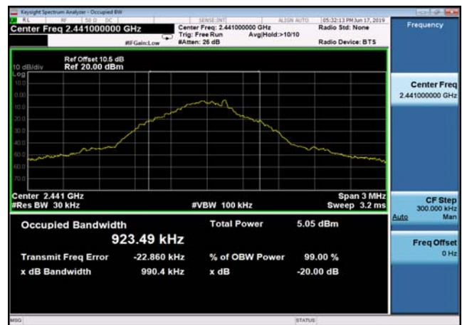
20dB Bandwidth: DQPSK,2402MHz,2DH5
