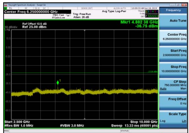
Conducted Emission: DQPSK,2441,2DH5 ,Band Edge HoppingOFF
