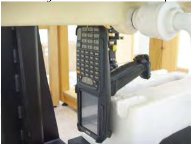
Fig.4 Bottom side of the EUT is paralleled and contact with flat phantom.
