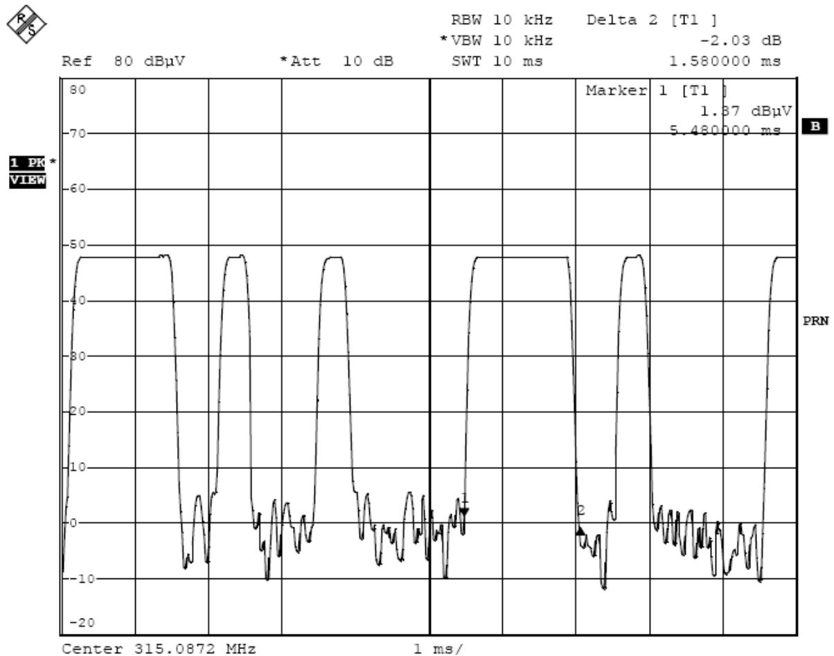
The graph shows the duration of long 'on' signal. From marker 1 to marker 2, duration is 1.58ms.
