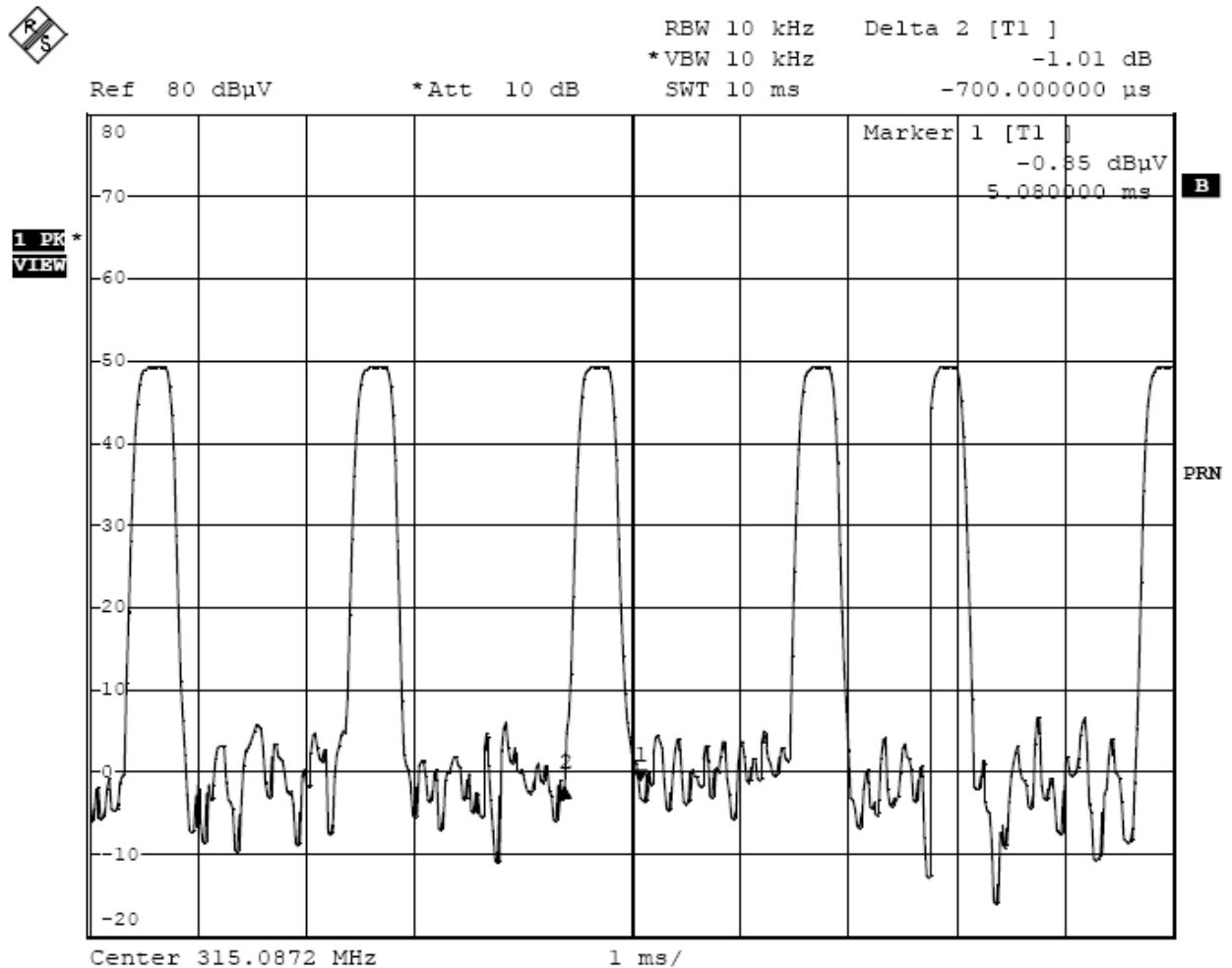
The graph shows the duration of short 'on' signal. From marker 1 to marker 2, duration is 0.7ms.
