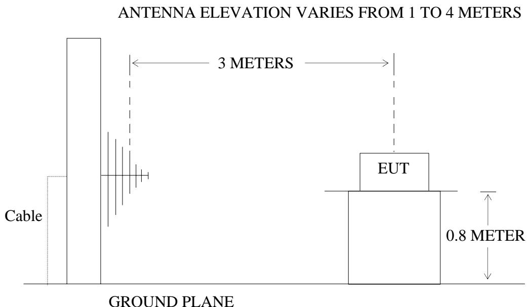
(EUT: Radio Frequency (RF) Repeater)
