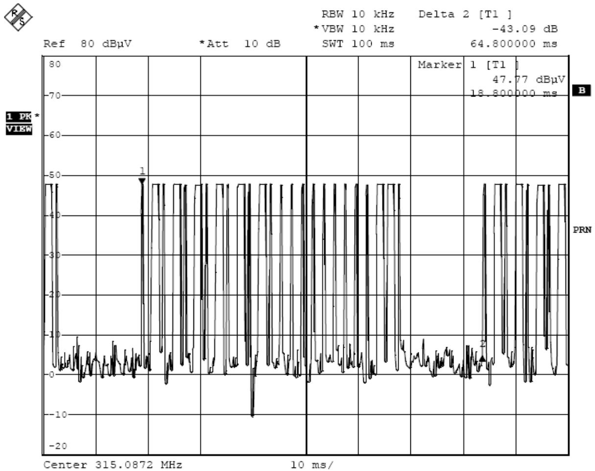
The graph shows the pattern of coding during the signal transmission. The time interval of one coding period starts from marker 1 to marker 2, Hence the total time of one period is 64.8ms. It sums of 8 long 'on' signals and 17 short 'on' signals.
