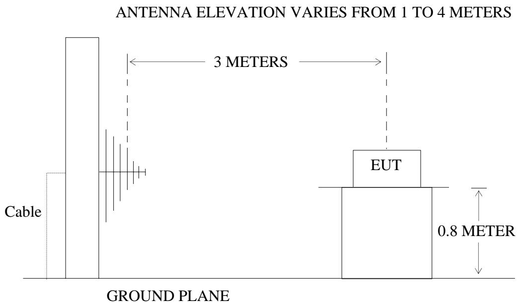
(EUT: Radio Frequency (RF) Repeater)
