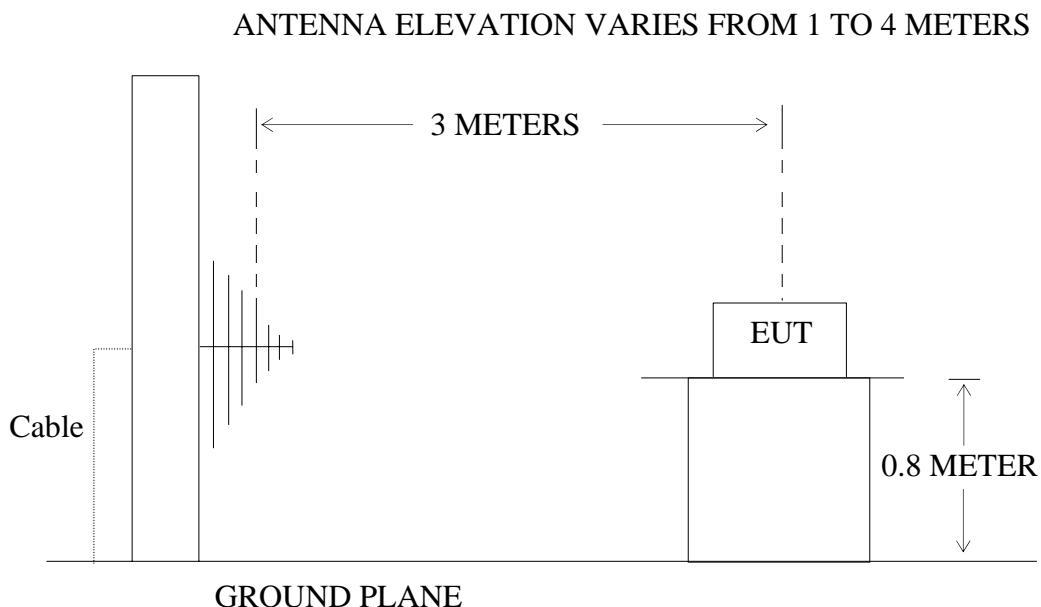
(EUT: Radio Frequency (RF) Repeater)
