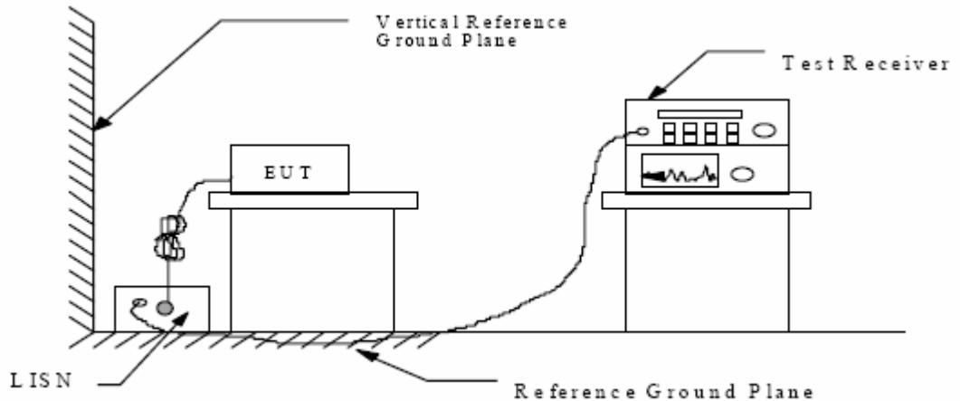
(EUT: Radio Frequency (RF) Repeater)
