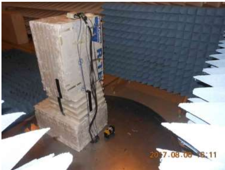
Radiated Emissions and Band Edge Above 1 GHz, 150cm table height
