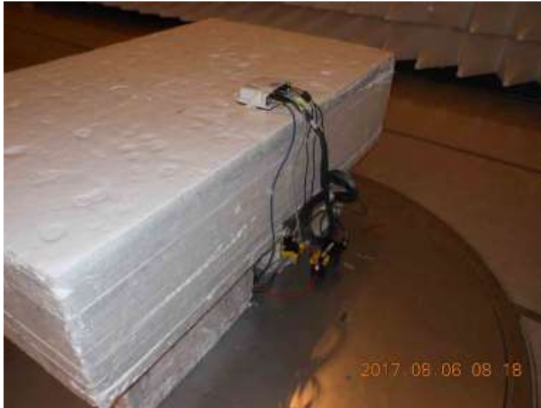
Radiated Emissions and Band Edge Below 1GHz, 80cm table height
