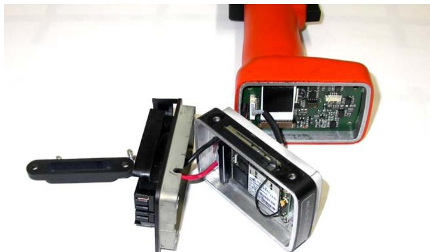
**Industrial cordless assembly Tool with WLAN data transmission**
