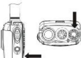
Press and hold the monitor button, rotate the volume control knob to adjust volume.
