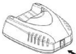
Put the output cable plug of charger adaptor into the jack, which is on the back of charger.
