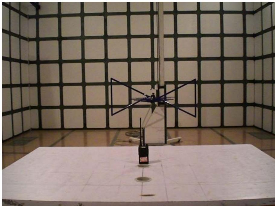
**Radiated Spurious Emission Setup 2(Above 1GHz)**
