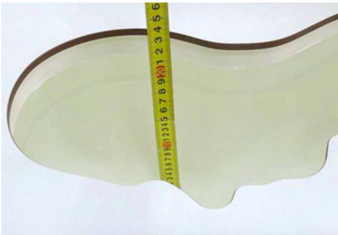
Picture 5: liquid depth in the head Phantom (1900 MHz, 15.1cm depth)
