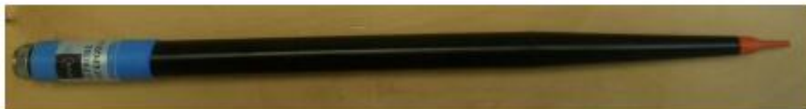
Figure 1 – MVG COMOSAR Dosimetric E field Dipole
