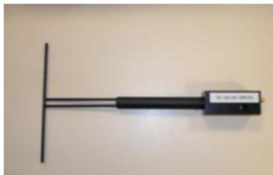
Figure 1 – Satimo COMOSAR Validation Dipole
