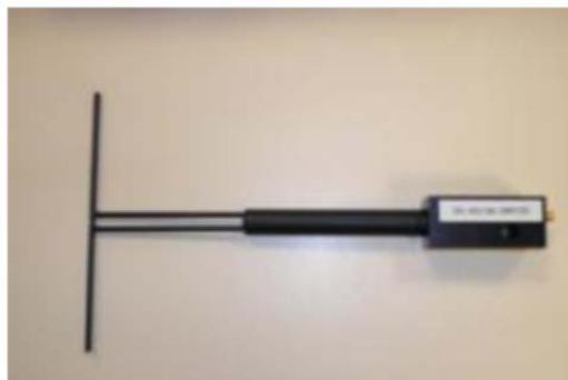
Figure 1 – Satimo COMOSAR Validation Dipole
