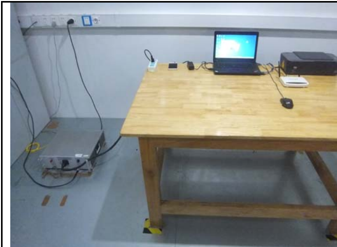
Conducted Emissions Test Setup – Front View
