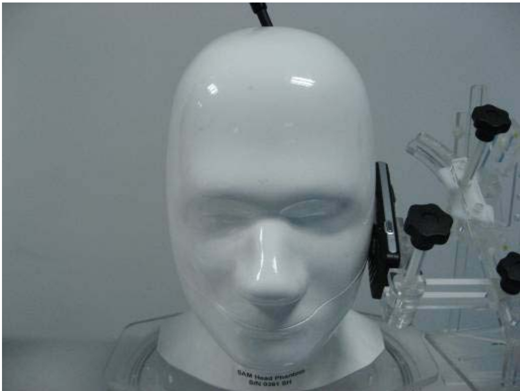
Fig.3 EUT Left Head Touch Cheek Position
