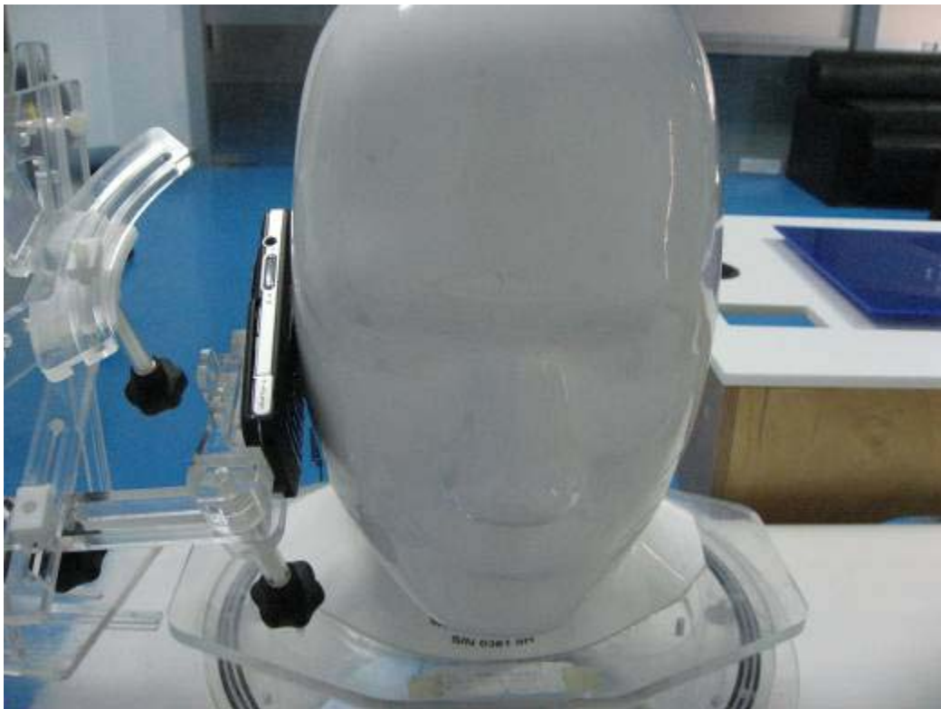
Fig.5 EUT Right Head Touch Cheek Position
