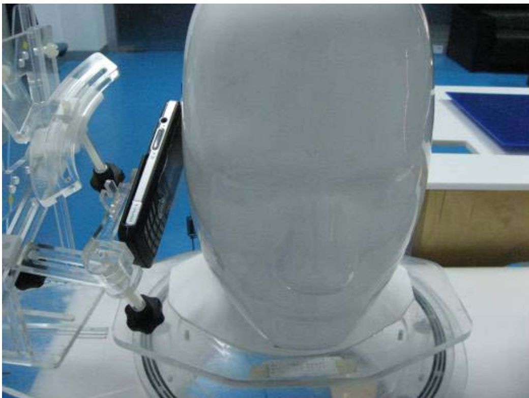
Fig.4 EUT Left Head Tilt15 Position
