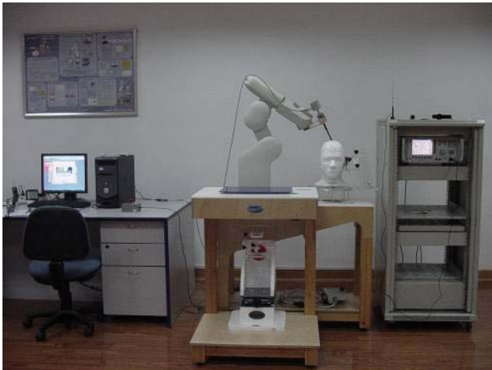
Fig.1 SARA2 System Test Layout
