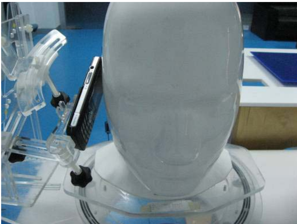
Fig.6 EUT Right Head Tilt15 Position
