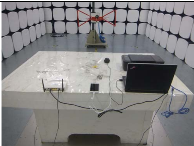
Radiated Emissions Test Setup Below 1GHz
