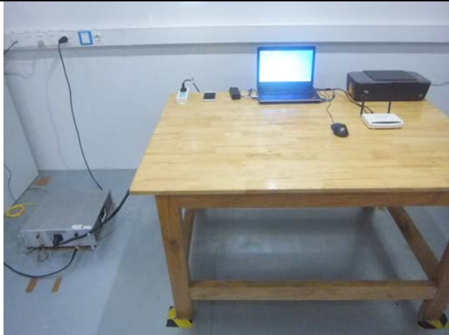
Conducted Emissions Test Setup – Front View
