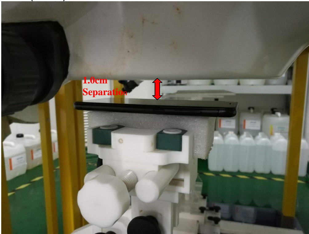
Body Setup Photo (LCD DOWN)
