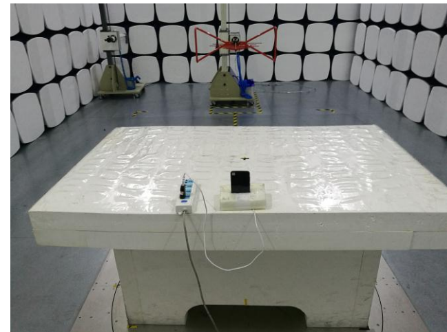
Conducted Emissions Test Setup Front View
