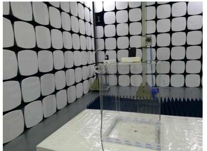
Radiated Spurious Emissions Test Setup Above 1GHz
