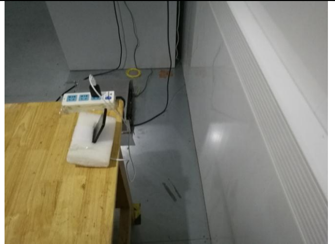
Conducted Emissions Test Setup Side View
