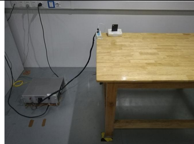
Conducted Emissions Test Setup Front View
