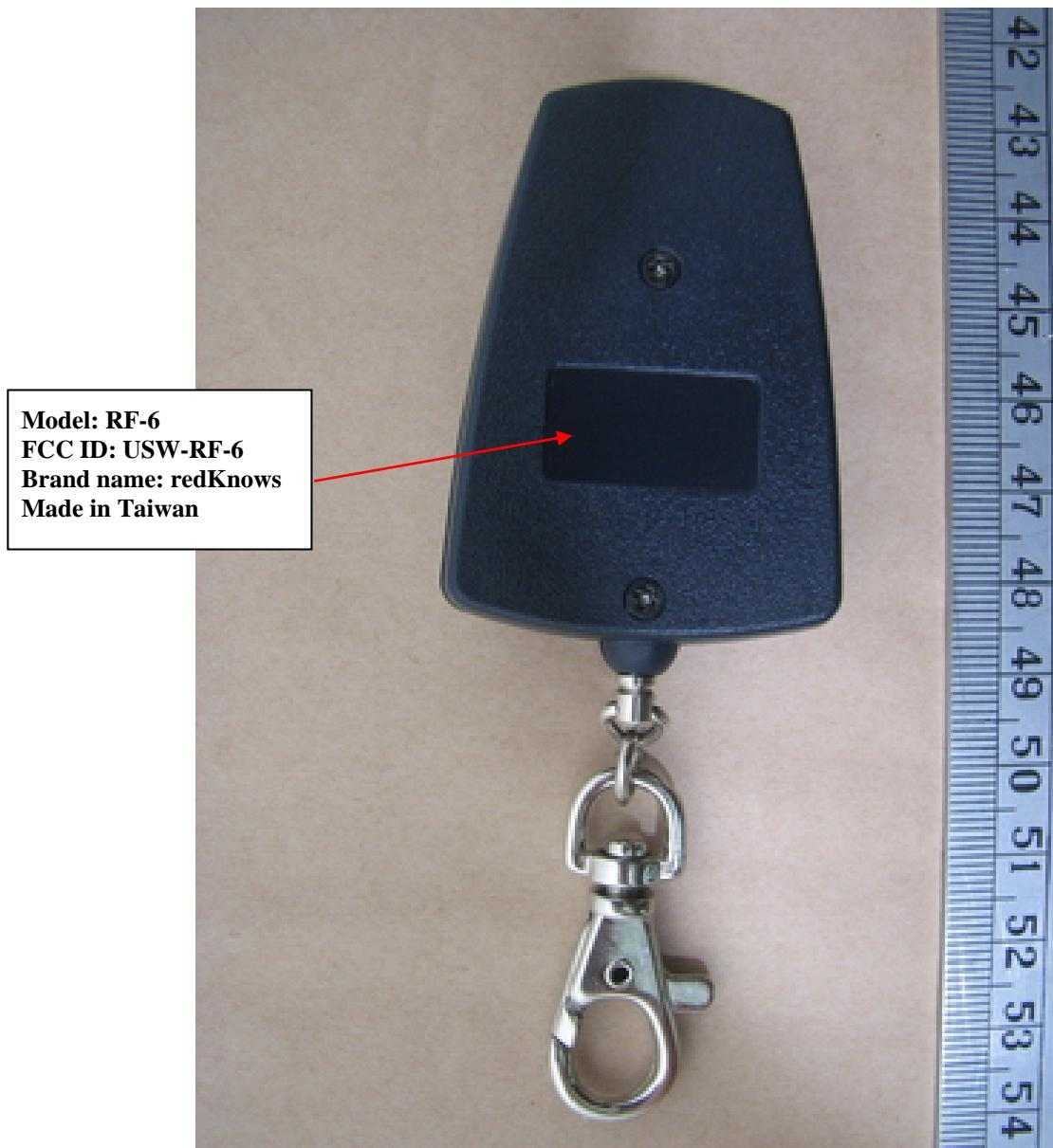
The label size is **19.5 mm X10 mm** and because of the size of this device is too small to be placed the other required statement, the following will be placed in the user's manual:
