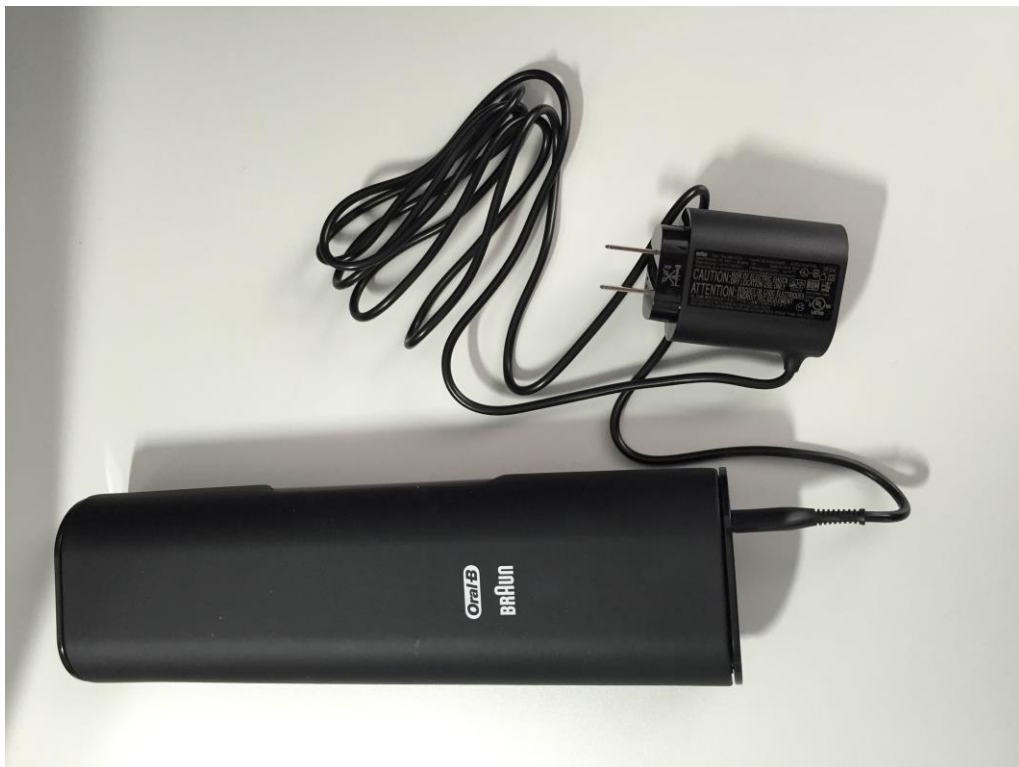
Picture 6: Charging travel case with power supply - top view
