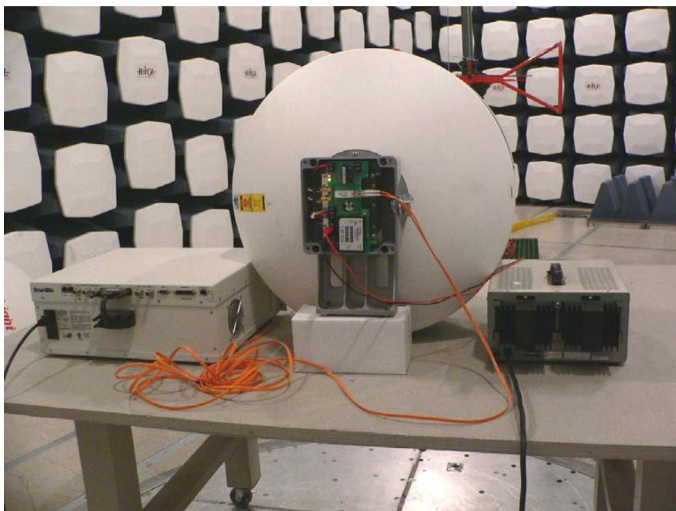
**11.3 (30 MHz - 1GHz) Radiated Emission 12 inches Antenna – Front View**
