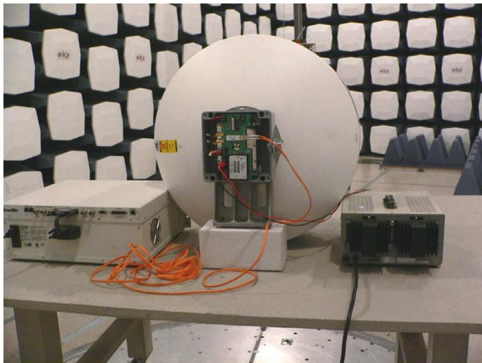
**11.7 (1 GHz – 20 GHz) Radiated Emission 12 inches Antenna – Front View**
