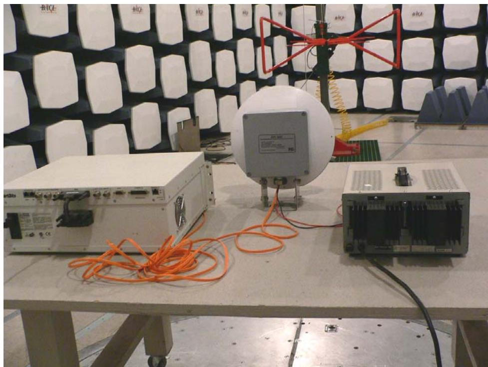
**11.5 (1 GHz – 20 GHz) Radiated Emission 24 inches Antenna – Front View**
