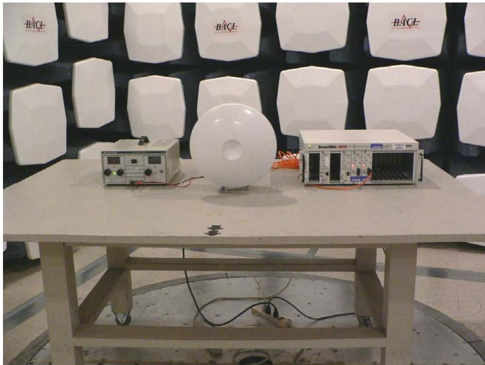
**11.8 (1 GHz – 20 GHz) Radiated Emission 12 inches Antenna – Rear View**
