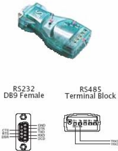
Figure3-8: RS485 to RS232C converter module
