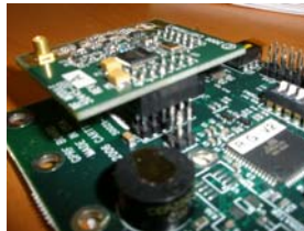
Figure 4: Proper Pin Alignment Figure 5: Proper Radio Installation
