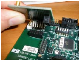
Figure 4: Proper Pin Alignment Figure 5: Proper Radio Installation
