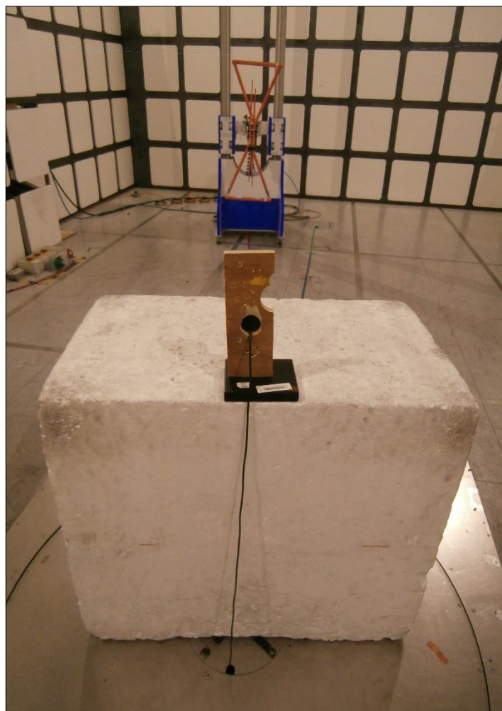
Figure 4 - Test Setup - 30 MHz to 1 GHz
