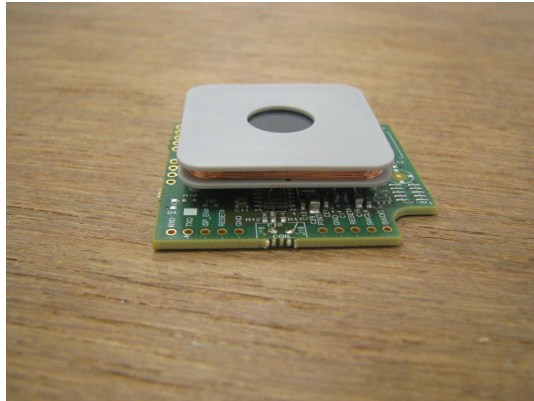
Reader module with antenna coil former
