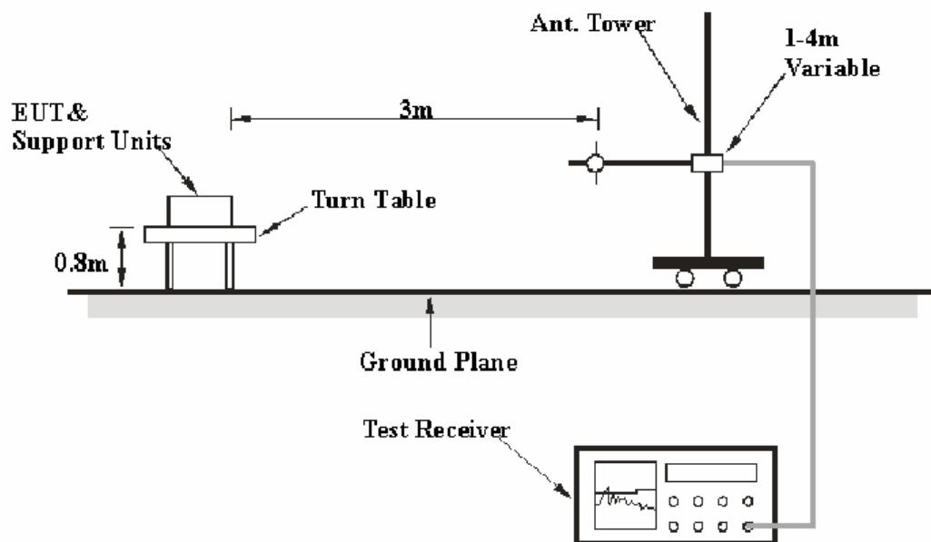
The radiated emission tests were performed in the 3 meters chamber B test site, using the setup accordance with the ANSI C63.4-2003. The specification used was the Part 15.205, Part15.209 and Part15.247 limits.
