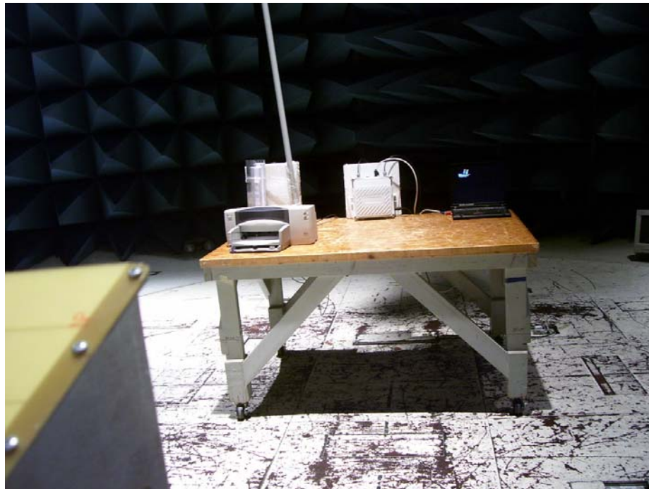
Photograph 4. Radiated Emission Limits, Test Setup, 1GHz- 2GHz
