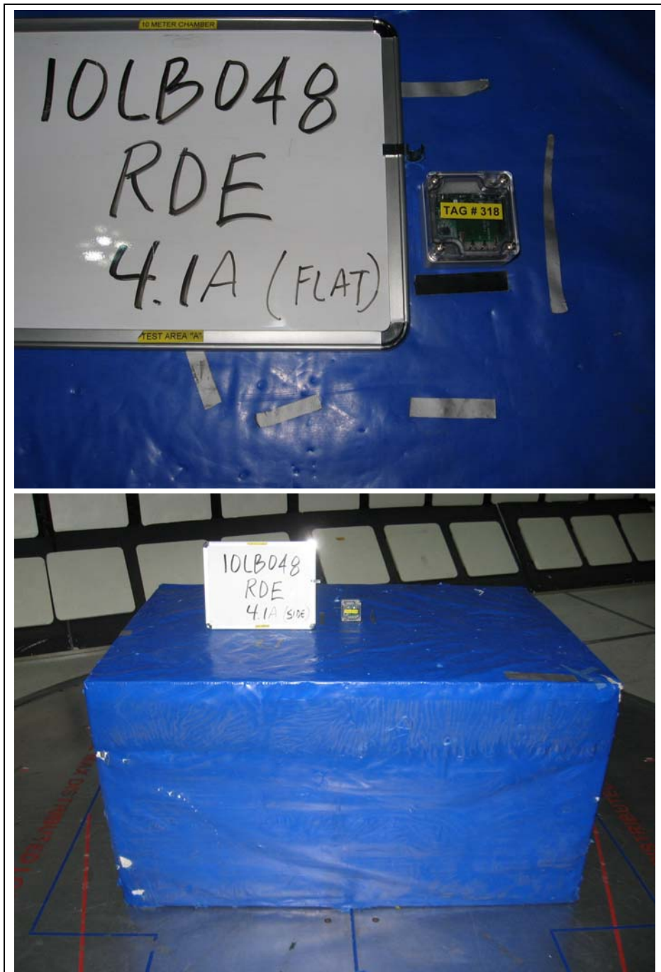
Figure 1 Test setup photo for Radiated Emissions (Tag #1, X-Y Orientation)
