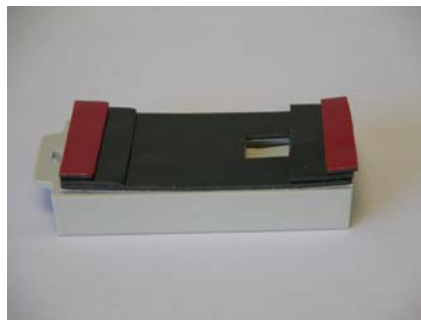
Building up adhesive to conform to curved substrates
