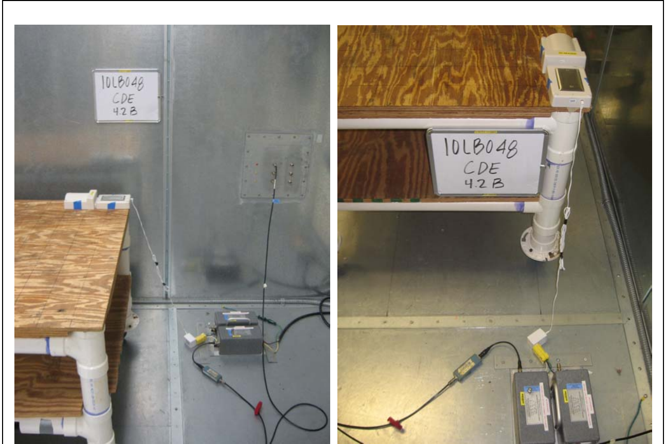
Figure 2 Test Setup for Conducted Emissions – DC Reader
