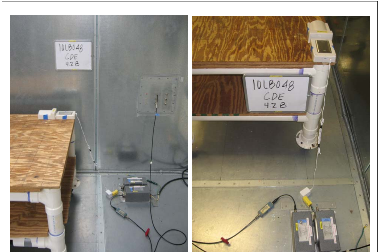
Figure 8 Test Setup for Conducted Emissions – DC Reader
