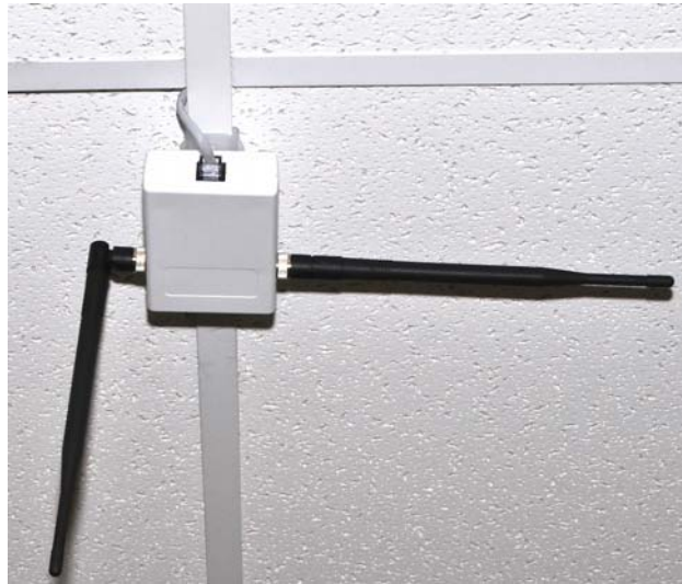
Fig 2 – Standard mounting for Remote Radio
