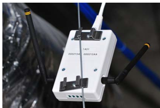
Fig 3 – Special mounting for Remote Radio on ceiling suspension wires
