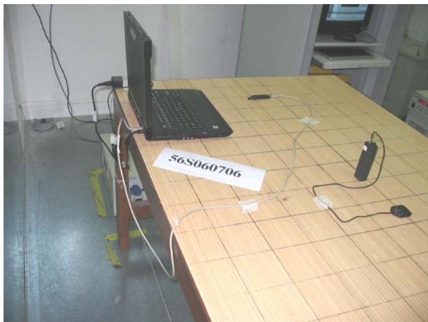
Conducted Emissions Test Setup (Rear View)
