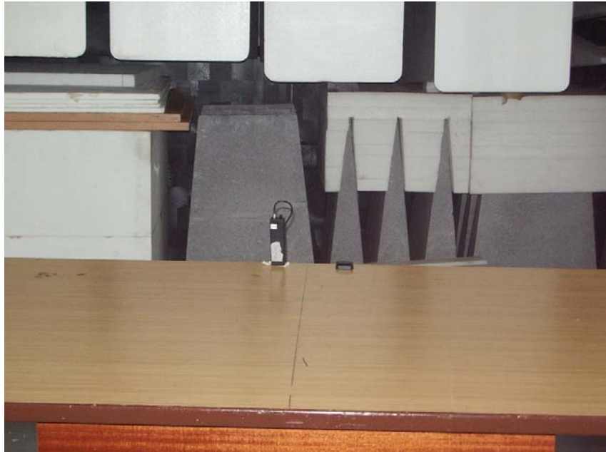
Radiated Emissions Test Setup (Front View) - Main Unit
