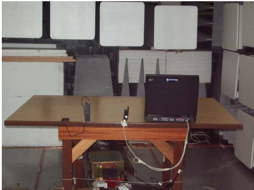
Radiated Emissions Test Setup (Rear View)
