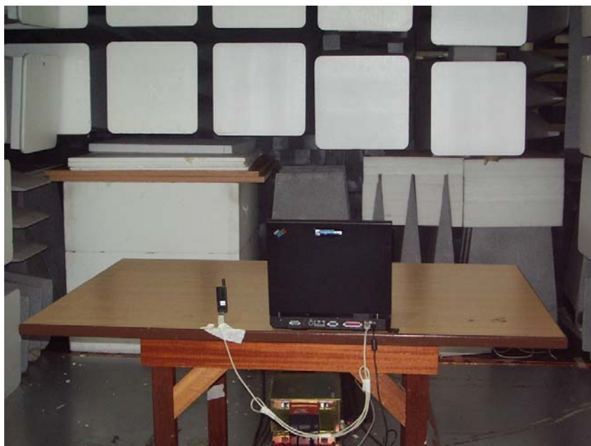
Radiated Emissions Test Setup (Rear View) ) - Remote Control Unit
