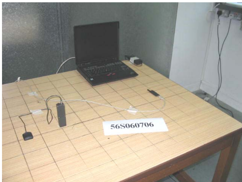
Conducted Emissions Test Setup (Front View)
