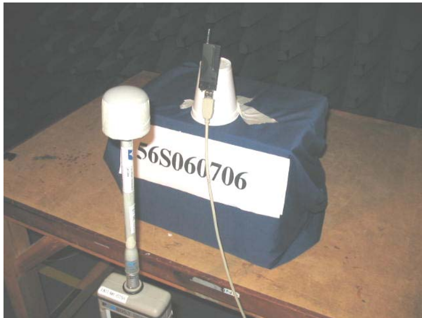
Maximum Permissible Exposure (MPE) Test Setup (Remote Control Unit)
