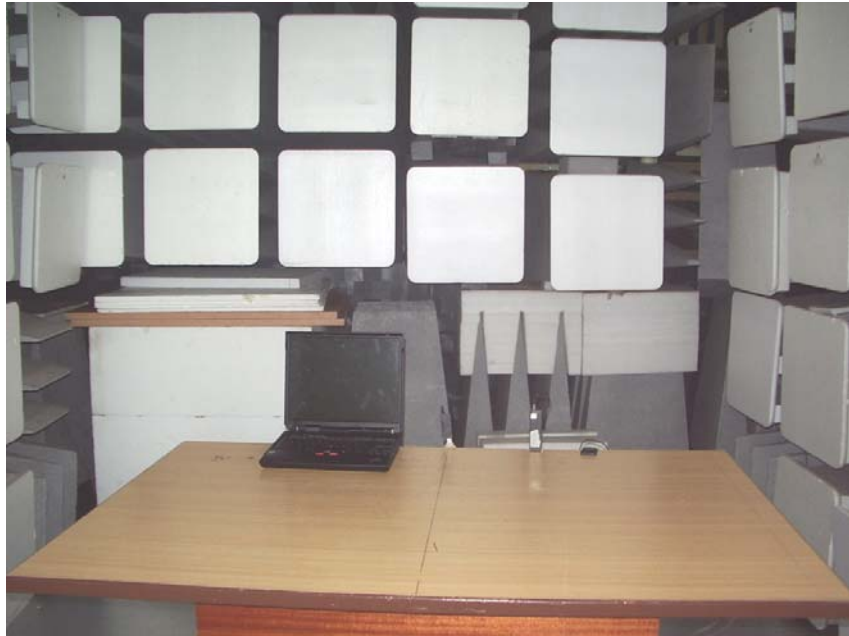
Radiated Emissions Test Setup (Front View)
