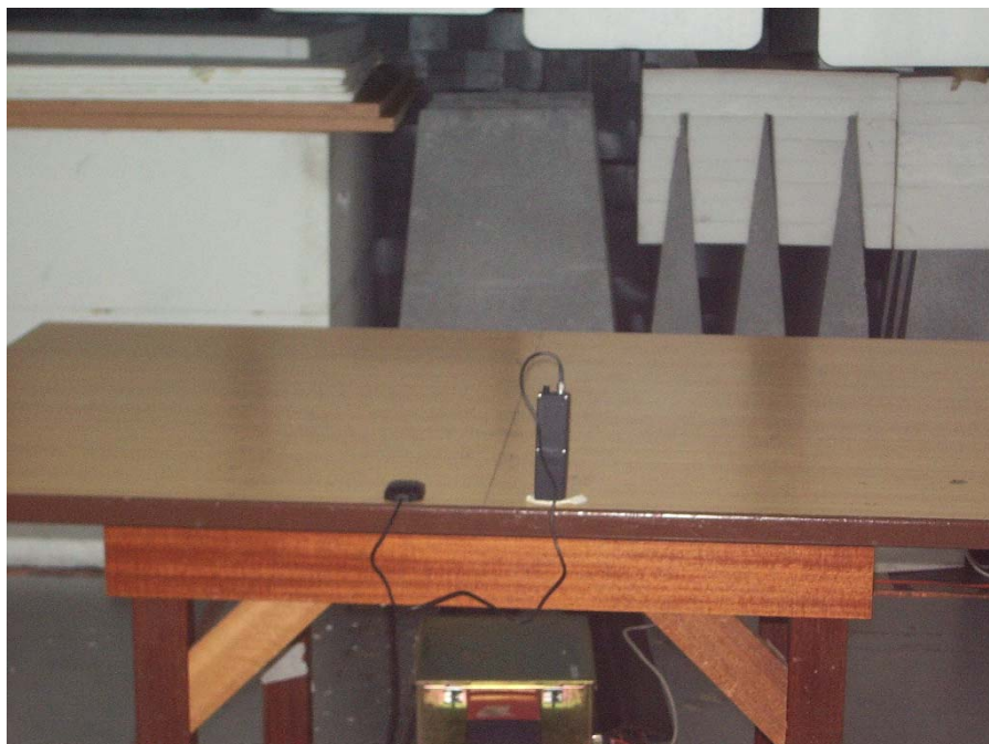
Radiated Emissions Test Setup (Rear View) ) - Main Unit
