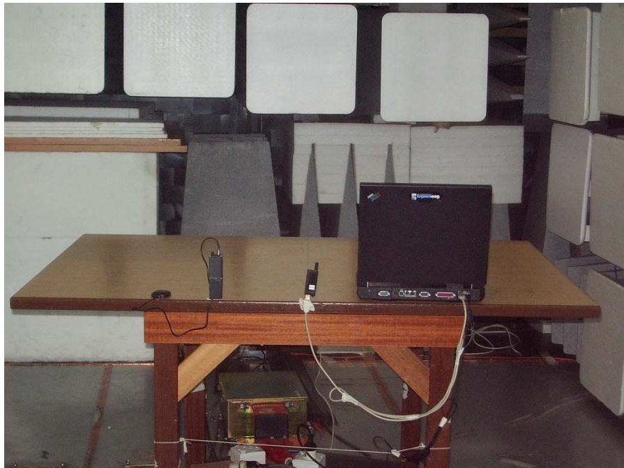
Radiated Emissions Test Setup (Rear View)
