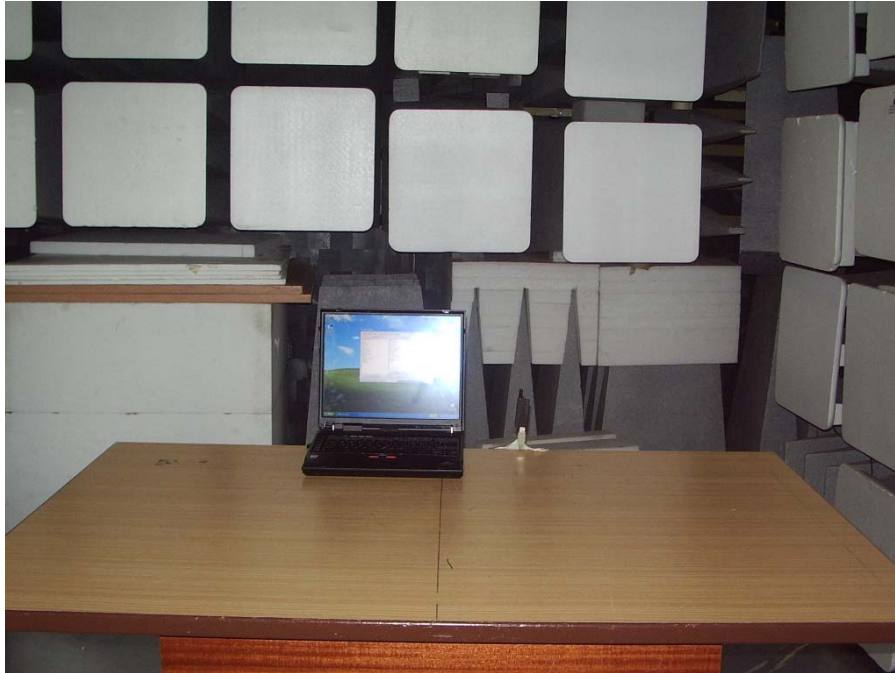
Radiated Emissions Test Setup (Front View) - Remote Control Unit
