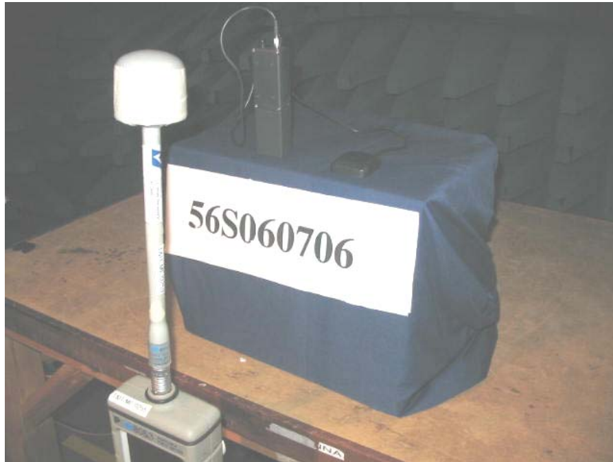
Maximum Permissible Exposure (MPE) Test Setup (Main Unit)
