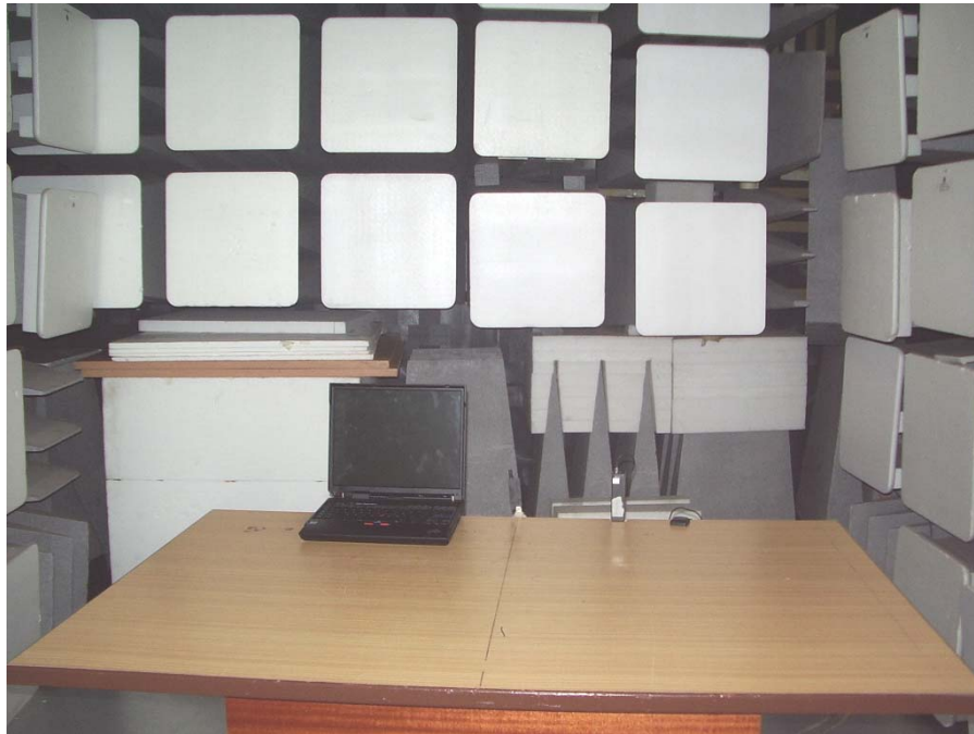
Radiated Emissions Test Setup (Front View)
