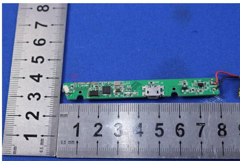
The antenna is integrated on the main PCB and no consideration of replacement. The best case gain of the antenna is 2.3dBi.
