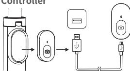
Take down the remote control, set a type-c interface at the bottom of the remote control, and connect Type-C to charge
