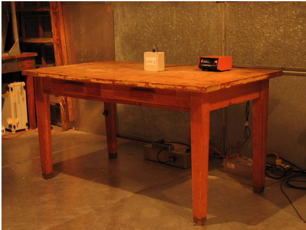
Conducted Emissions Test Setup
