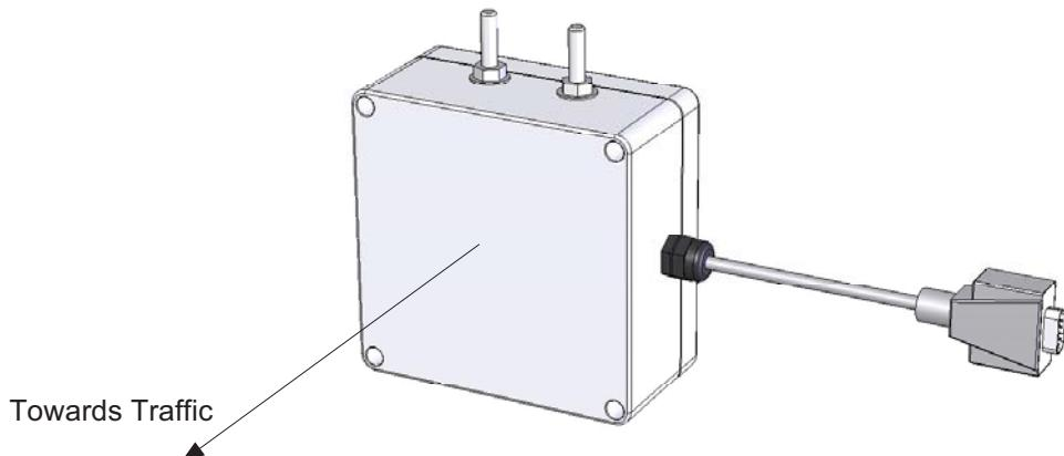
The unit has a configurable dip switch. In most cases it will not be necessary to change it, but in rare instances it could be necessary. Remove the lid of the unit to expose the underlying circuit board that contains the dip switch. See the following figure.
