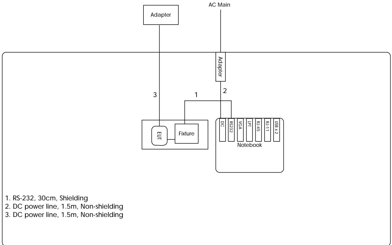
A test fixture is used to set EUT in CTX mode. The spurious emission above 1 GHz is independent of the accessories.
