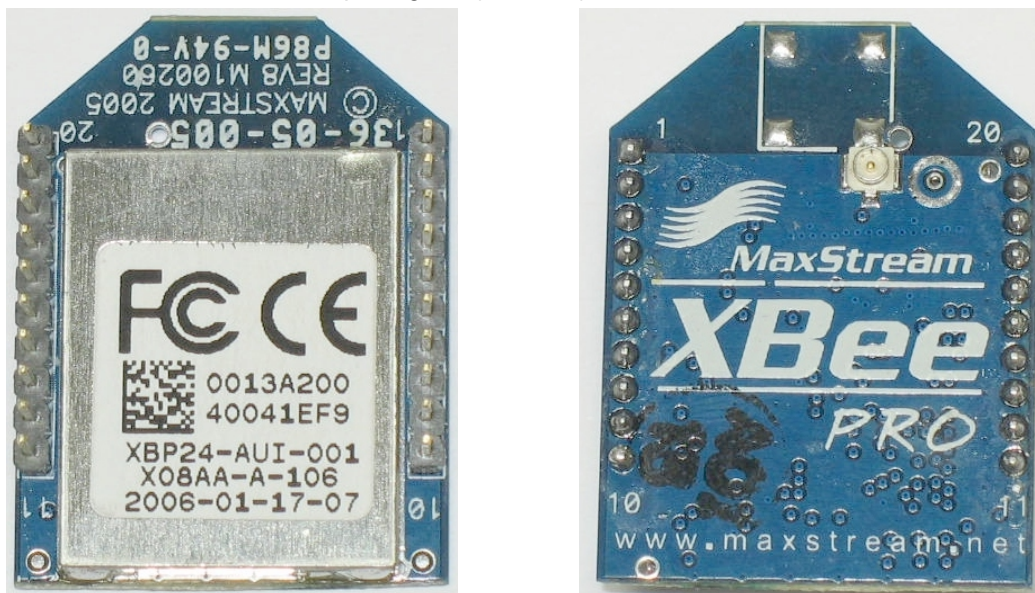
Max Stream XBee-pro ZigBee (802.15.4) Transmitter, XBP24-AUI-001 on the PDA Interface Board
