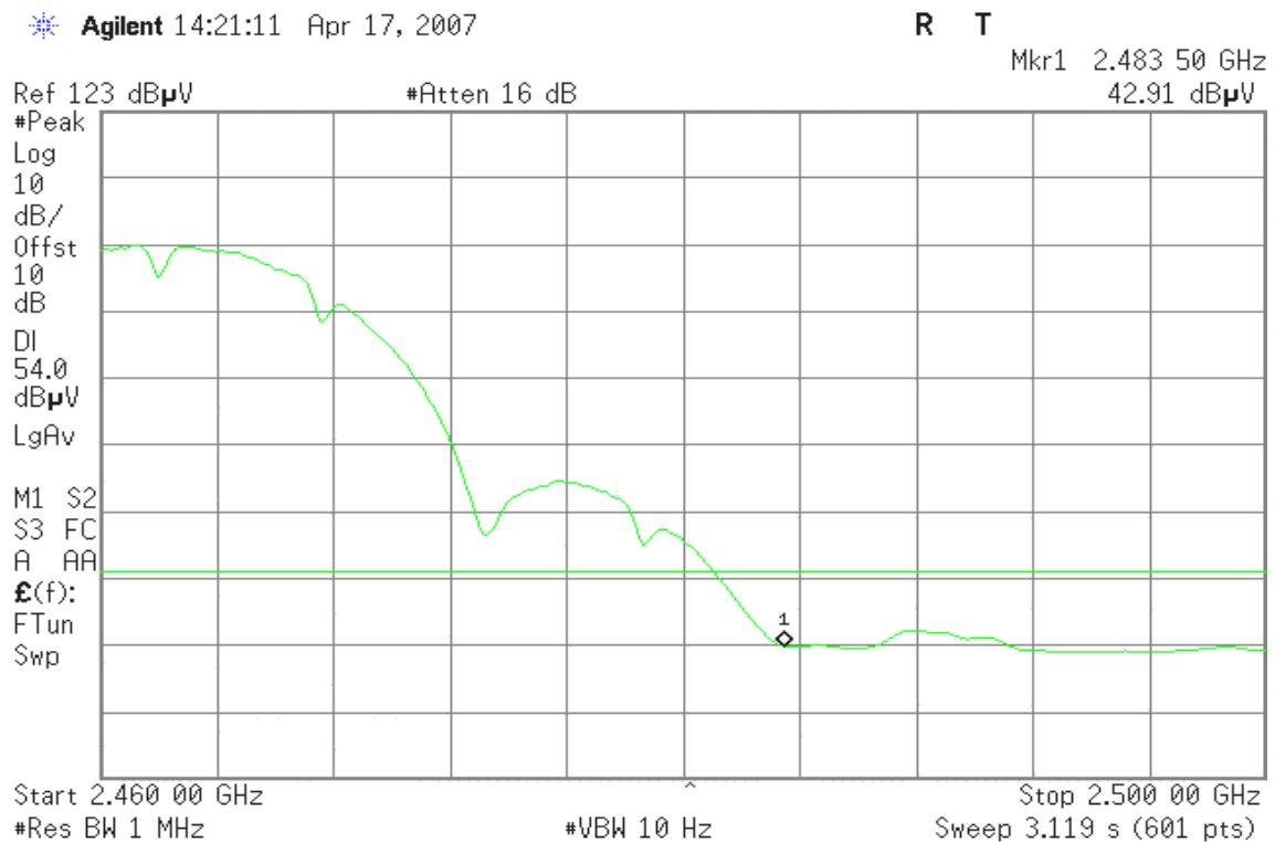
**Band Edges (IEEE 802.11g / CH Low)****Detector mode: Peak****Polarity: Vertical**
