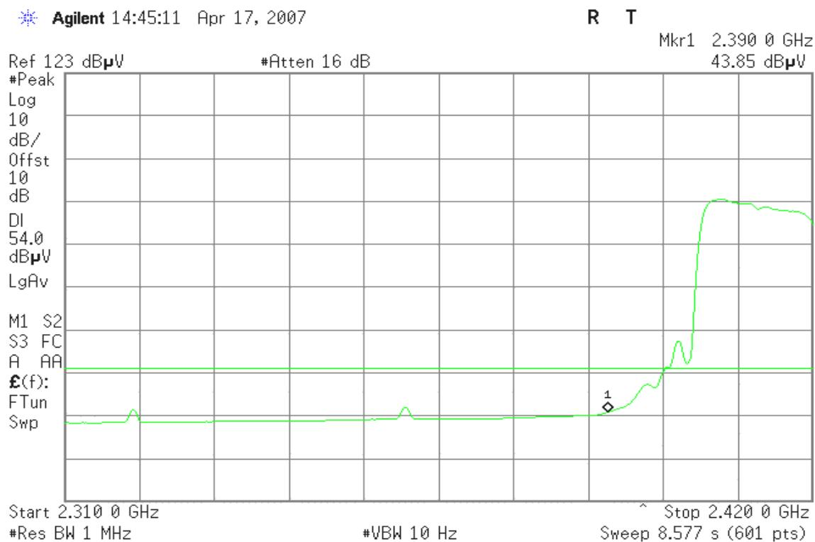
**Band Edges (IEEE 802.11g / CH High)****Detector mode: Peak****Polarity: Vertical**
