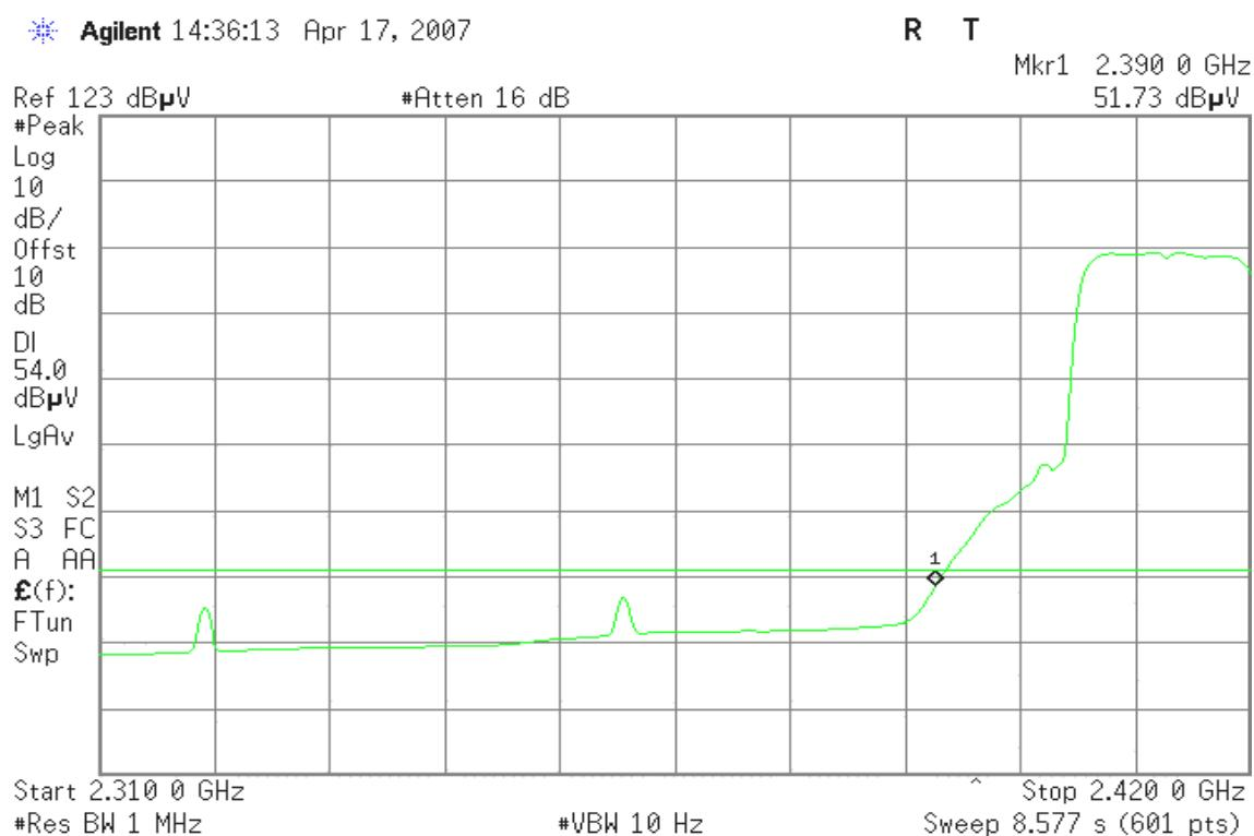
**Detector mode: Peak****Polarity: Horizontal**
