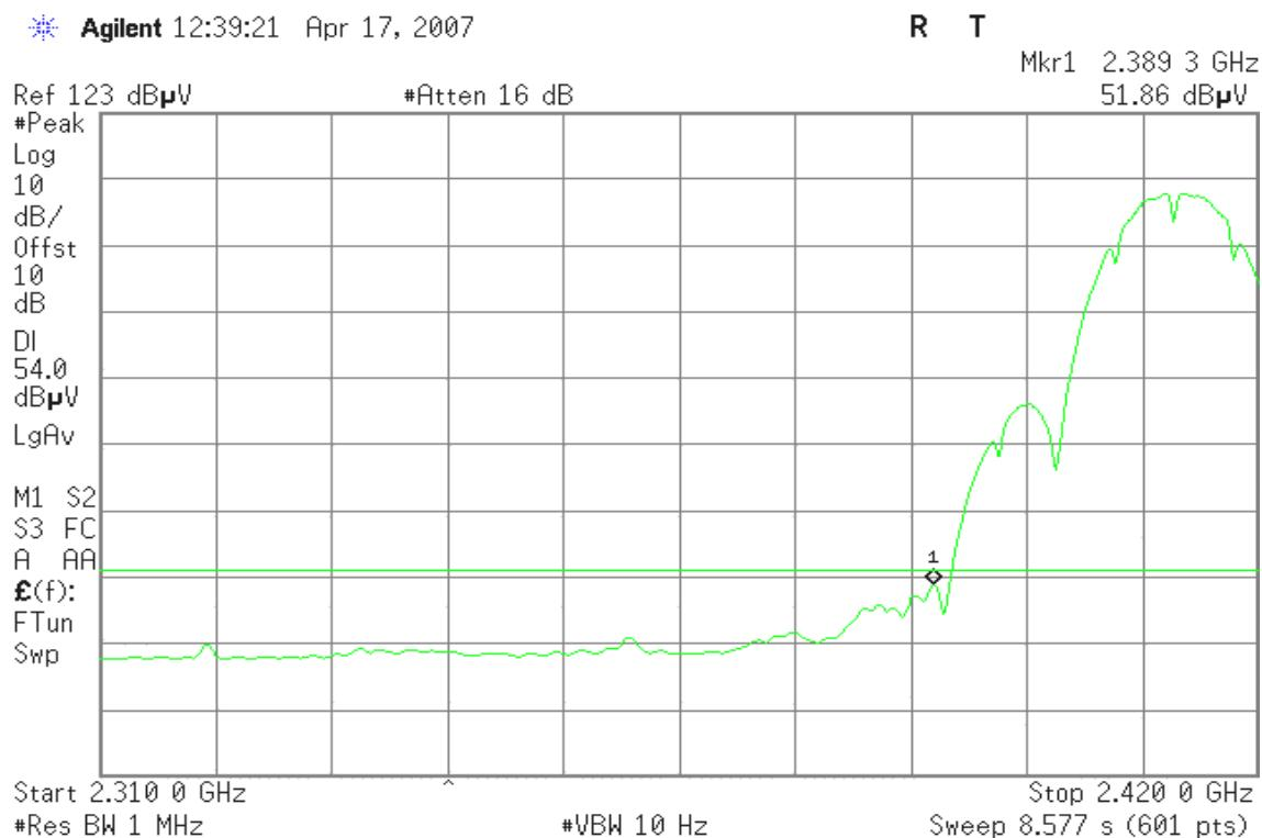
**Detector mode: Peak****Polarity: Horizontal**
