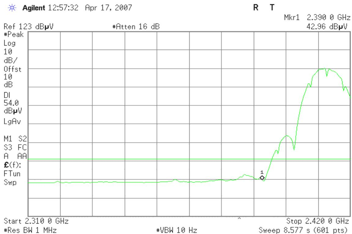
**Band Edges (IEEE 802.11b / CH High)****Detector mode: Peak****Polarity: Vertical**
