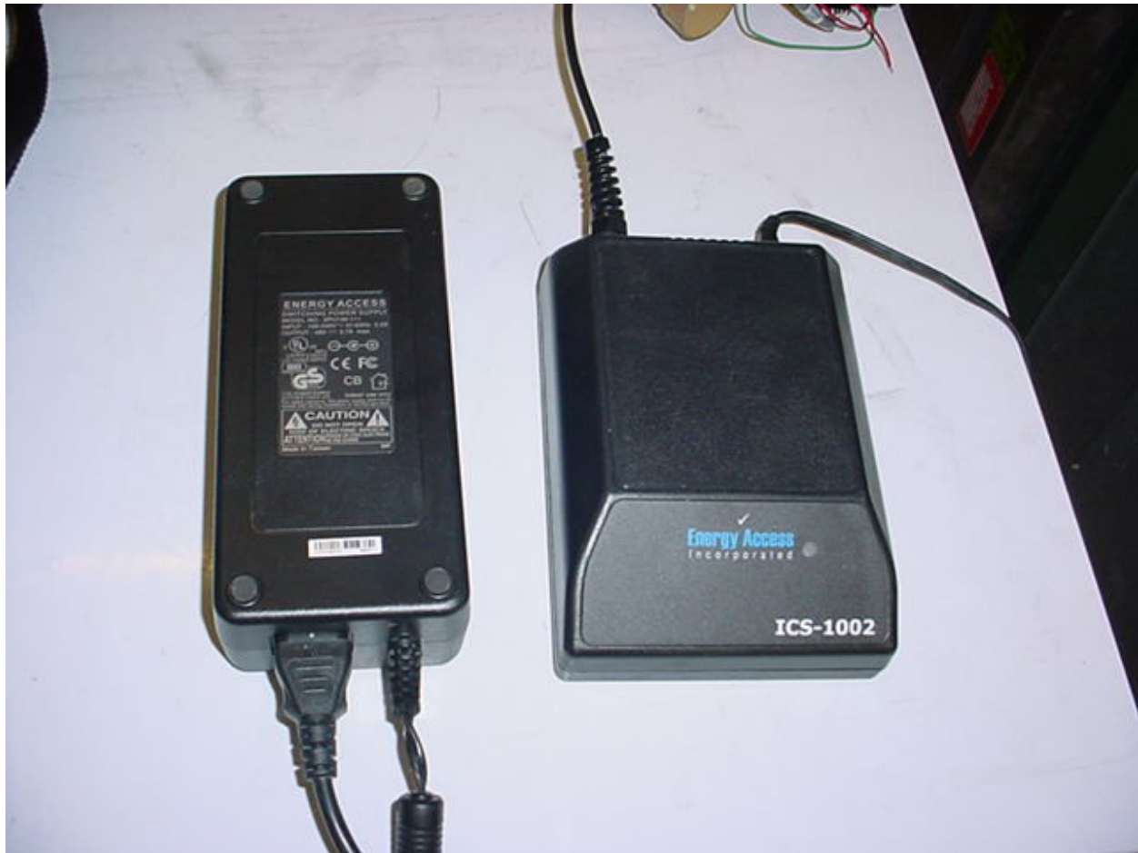
Power Supply and Battery Charger
