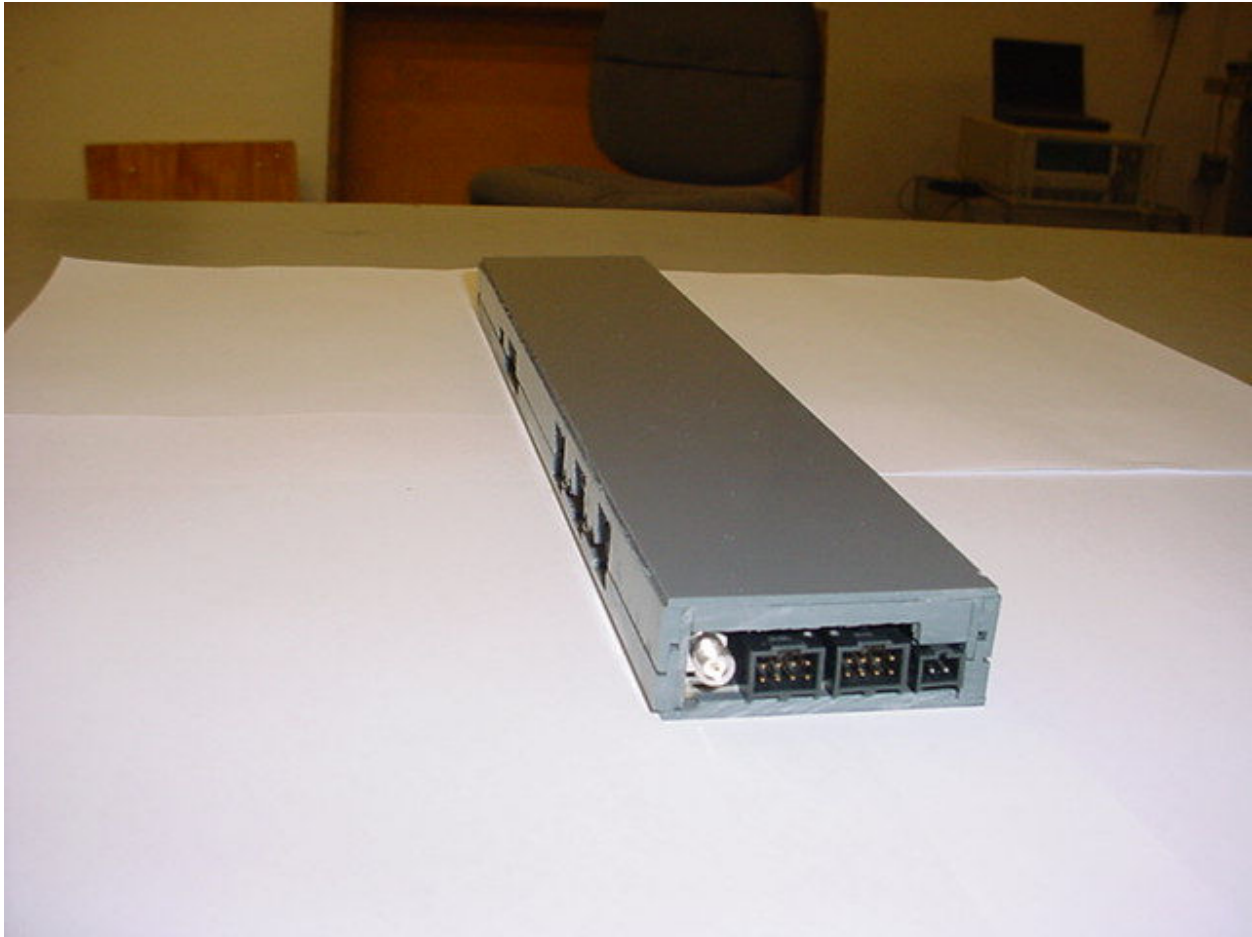
Side View (antenna, power, magnetic switches connectors)
