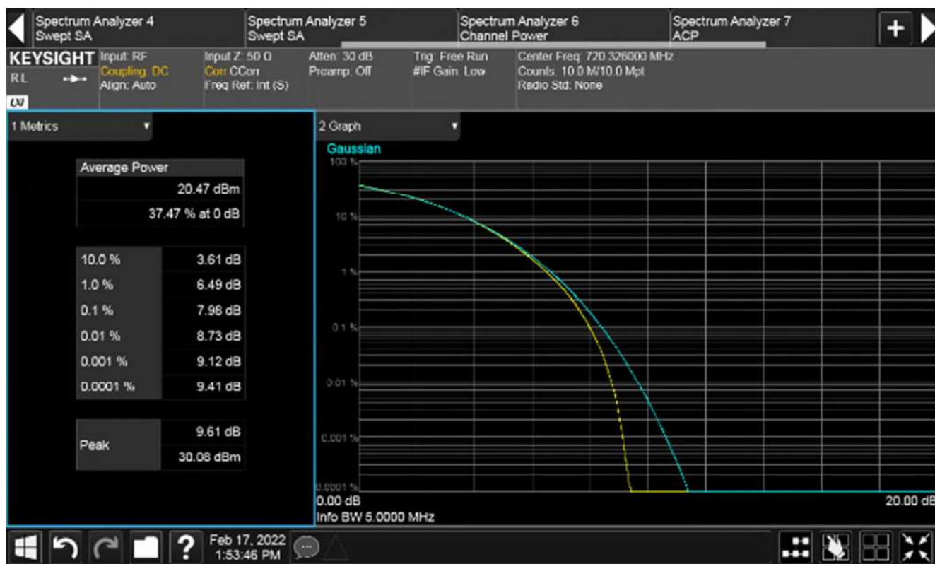
Plot of Peak to Average power ratio at determined f_0 in band 716-758 MHz
