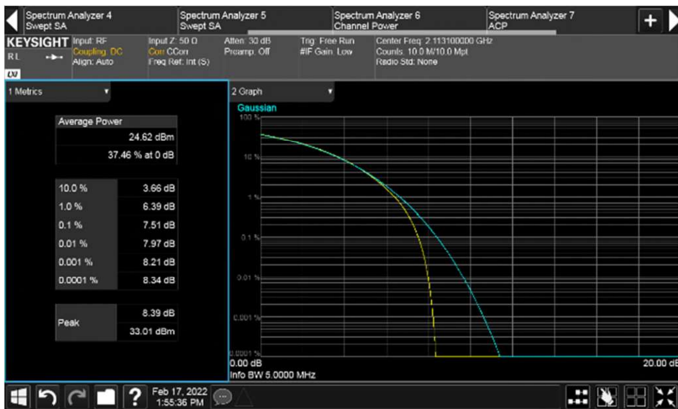
Plot of Peak to Average power ratio at determined f_0 in band 2110-2200 MHz
