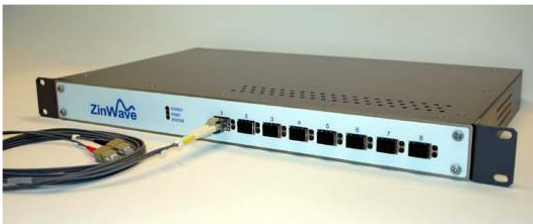
Figure 3-1: ZinWave 2700 Hub Unit with 8 ZinWave 2780 modules
