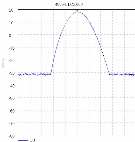
Centre 1.93125 GHz; Span 20.0 MHz
