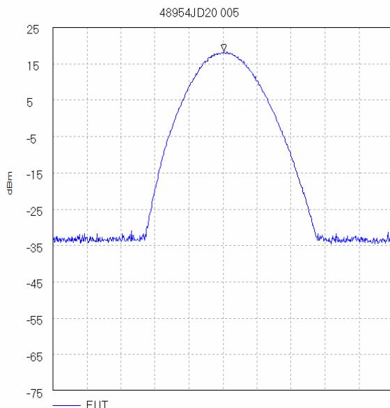
Centre 869.7 MHz; Span 20.0 MHz
