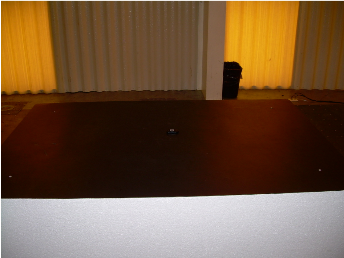
Photograph 3 - View of the Radiated Emission Test Setup (Horizontal Flat Alignment)
